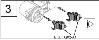
4 Notice the presence of the O-rings before placing a pilot cartridge
