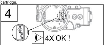
5 Place the pilot cartridge and fasten the screws according to the sequence, with a Phillips head no. 2 screwdriver.
