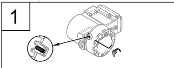
2 Unlock the switch cartridge turning the screw 90° with screw driver 0.8 X 4.0 Max.
