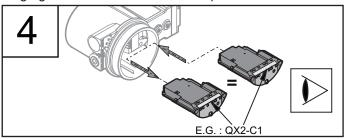
5 Notice the position of the pin before replacing a switch cartridge.
