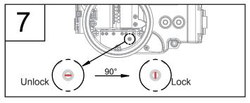
8 After switch cartridge replacement, mount and lock the cover to the module.
