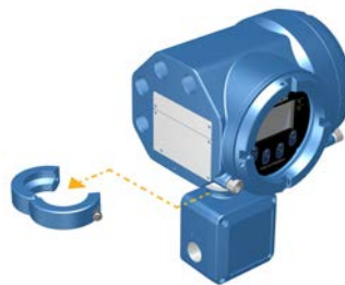
Figure 3-18: Removal of the clamp
