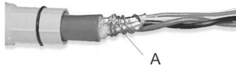
A. Drain wires wrapped around shield
