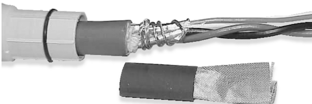
Shield drain wire(s) wrapped twice around exposed shield foil
