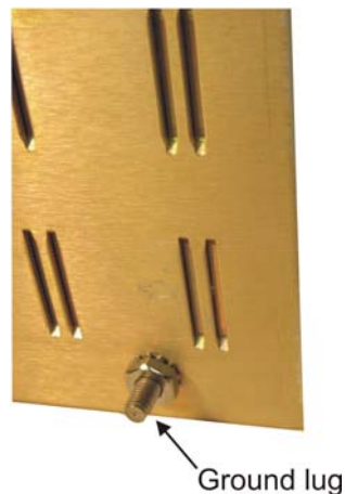
Figure 2-4. Ground Lug on Bottom of Chassis
