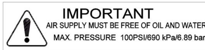
Figure 1.2 Caution label on the 2000X ae Actuator for the factory air supply
