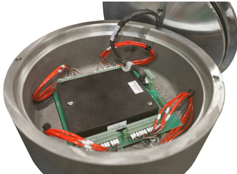
Figure 3-17: Rosemount 3418 Ultrasonic meter acquisition connection board wiring
