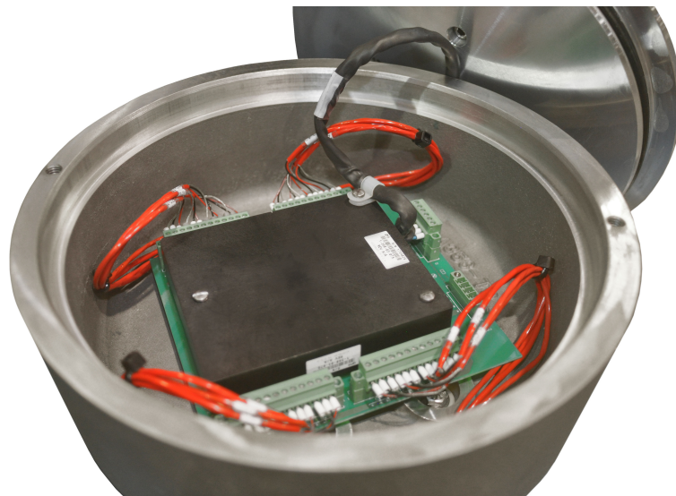
Figure 3-16: 3410 Ultrasonic Meter acquisition connection board wiring
