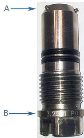
Figure 3-6: Transducer holder length and set screw identification
