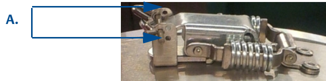
Figure 3-16 Shroud latch holes for security wire seals
