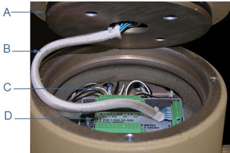
Figure 3-31: Acquisition Module cable and transducer wiring
