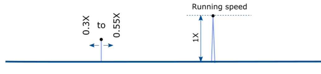
Figure 3-7: Spectrum – oil whirl
