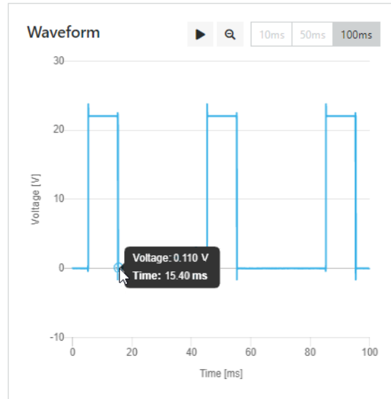
Figure 6-11: End of the period portion smaller than or equal to 50% (Point 3)
