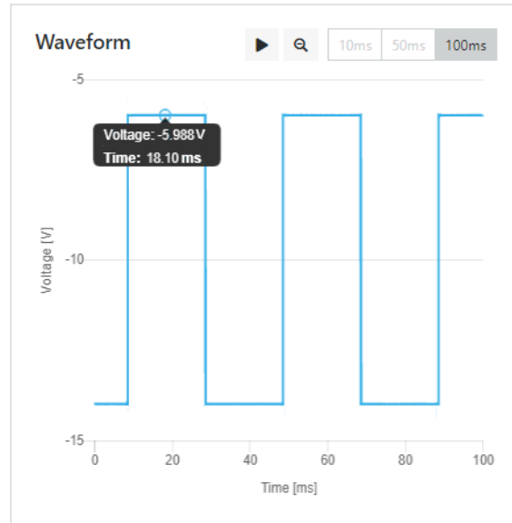
Figure 6-13: Upper voltage and DC level of a negative input signal
