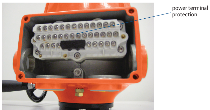
Figure 13 Overview of the cable entry conduits
