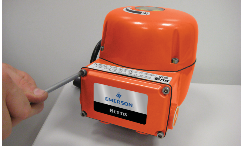
Figure 9 Removal of the terminal board enclosure
