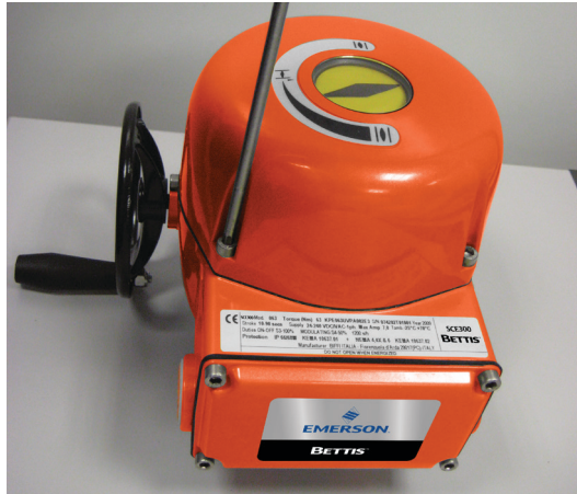
Figure 14 Removal of the control unit cover
