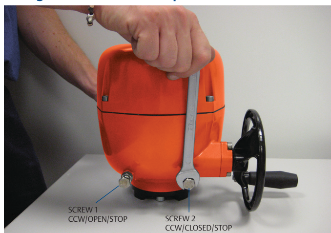
Figure 8 Setting of the Mechanical Stop
