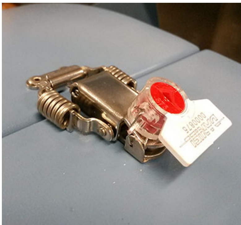
Figure 3-33: Shroud latch with Security seal
