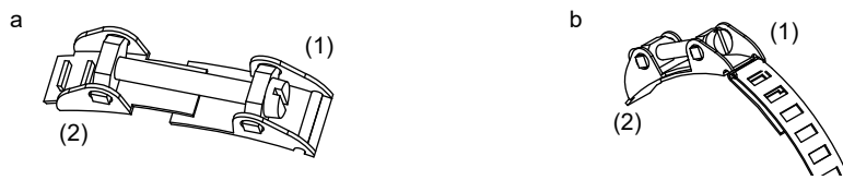
Fig. 6.70: Temperature probe on the pipe
