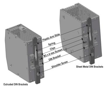
2. Retain / Slide the two DIN brackets back of the unit. Place the Panel Mount Bracket on top of the DIN Brackets. Use the DIN Bracket to align the Panel Mount Bracket in the mounting hole. Fixed the Panel Mount Bracket using the M3 x 8mm Phillip screw. Recommended torque is 6lbf-in (7kgf-cm).
