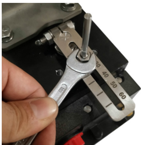
Figure 5-19 Installing the Dowel Pin
