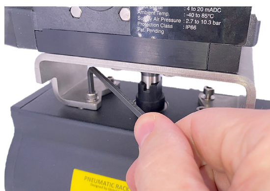
Figure 5-7 Tightening the Bracket Bolts
