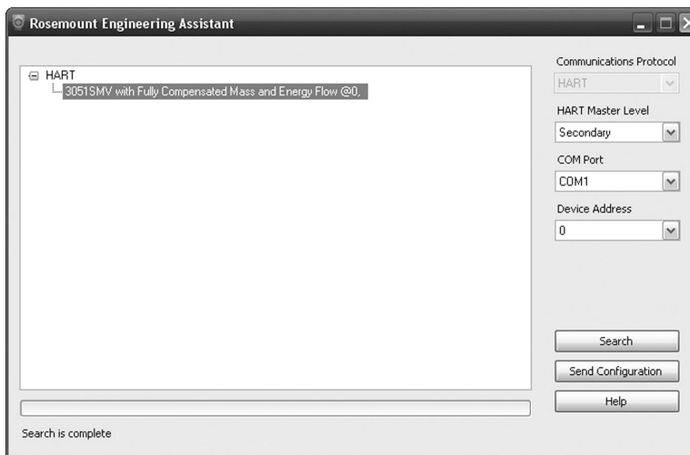
Figure 2-12: Engineering Assistant Device Connection Screen
