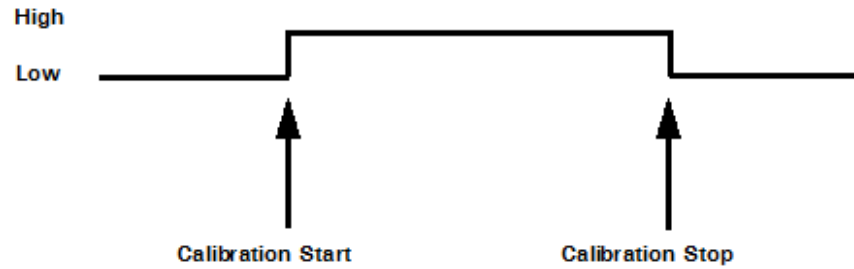
Figure 4-13: Gating configuration parameter State gated, active high
