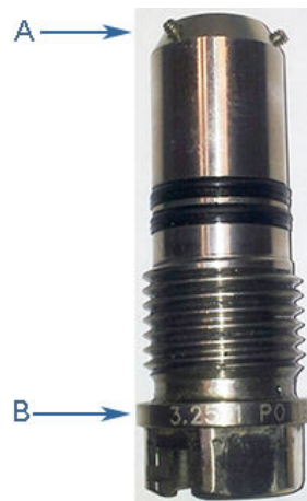
Figure 3-6: Transducer holder length and set screw identification
