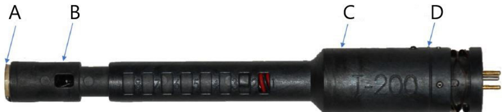
Figure 3-10: T-200 transducer capsule assembly
