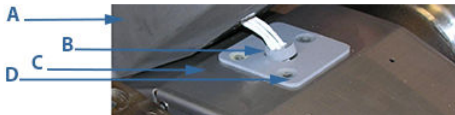
Figure 3-28: Split shroud transducer cable seal and gasket
