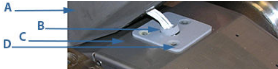
Figure 3-37: Upper shroud feed-thru cable seal
