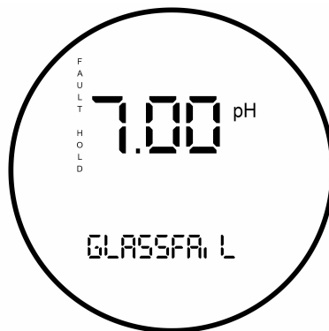
Figure 8-7: Disabling Fault Annunciation
