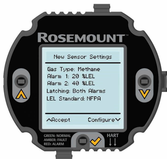
Figure 3-23: New Sensor Detected Screen
