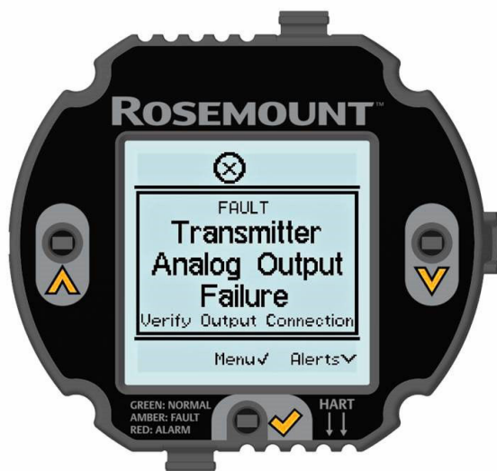
Figure 3-26: Current Loop Fault Screen
