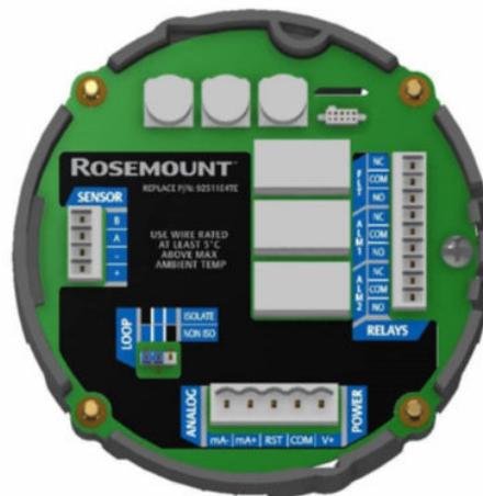
Figure 3-3: 925 Transmitter Terminal Block
