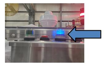
Press and Hold the Green Button until no longer flashing (approximately 3-5 seconds). An alarm will sound, the status indicator light will go green and the conveyor will start.
