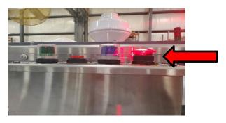
Press the BLUE flashing light until solid blue; the green light will flash
