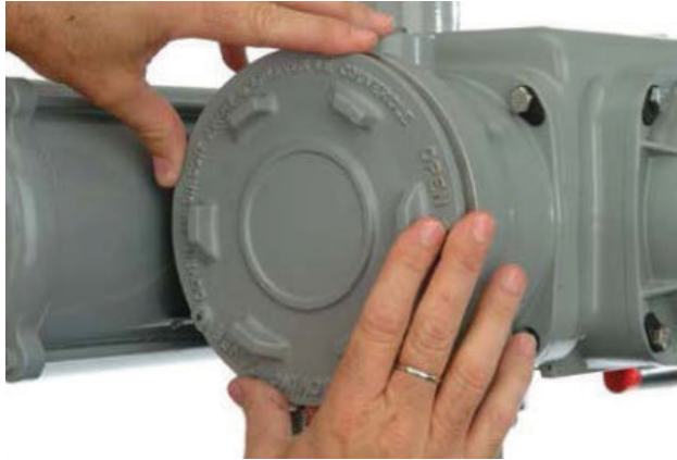
Figure 8 Remove STC Cover Turning Counterclockwise
