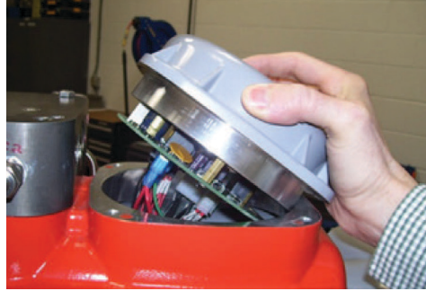
Figure 19 Remove Cover for Limit Switch Chamber
