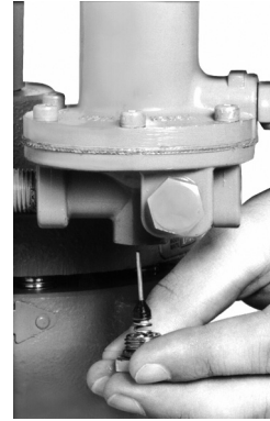
Figure 11. 161EB Series Pilot Trim Removal/Installation
