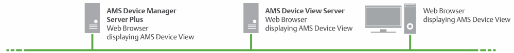
Figure B-2: AMS Device View server not on an AMS Device Manager Station
