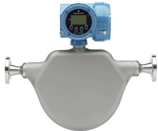
Micro Motion ELITE CMFS with 5700 Transmitter, which can calculate the real-time gas standard volume of natural gas with external specific gravity or base density input from the SGM
