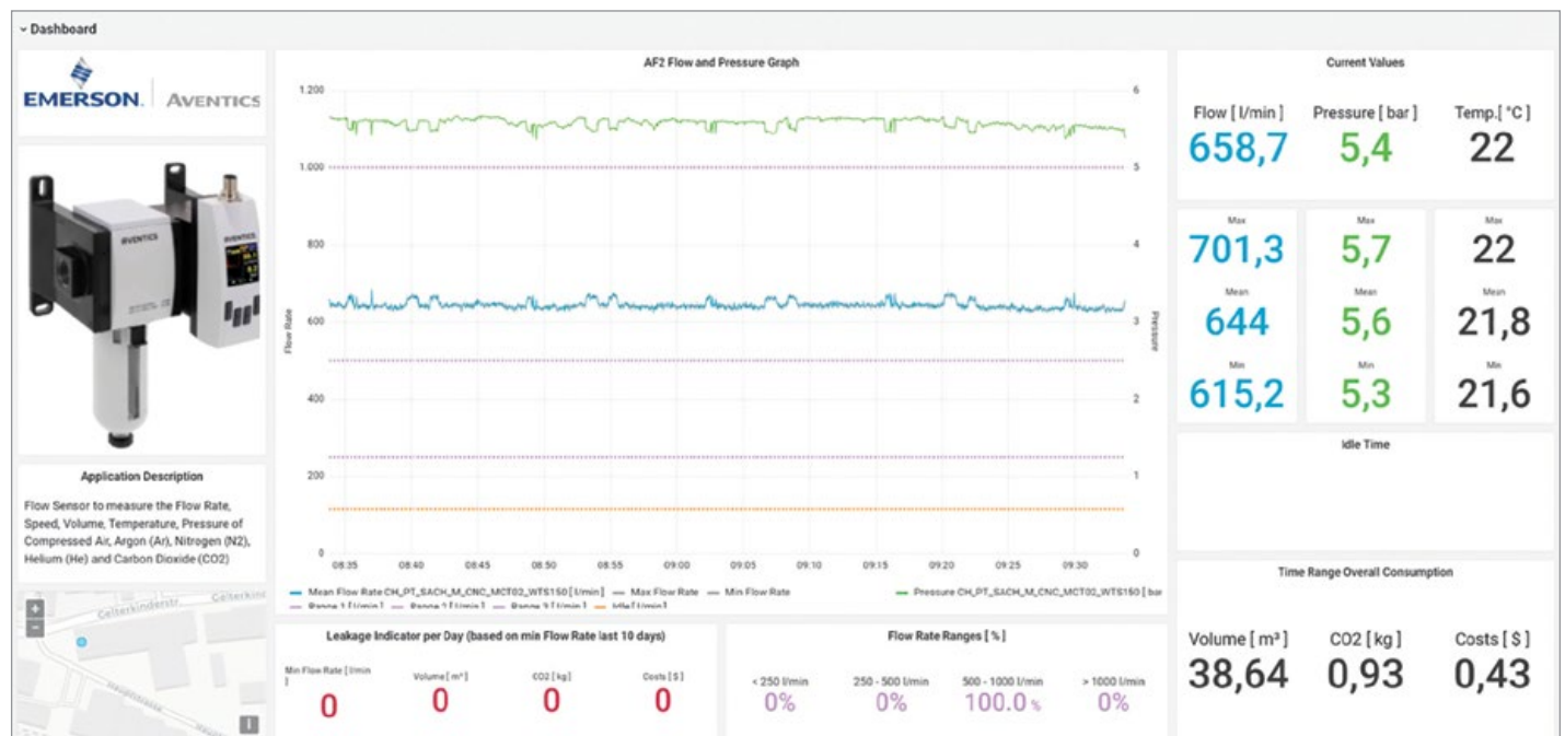
The AF2 dashboard measures flow rate, speed, volume, temperature and pressure. Image courtesy of Emerson.
