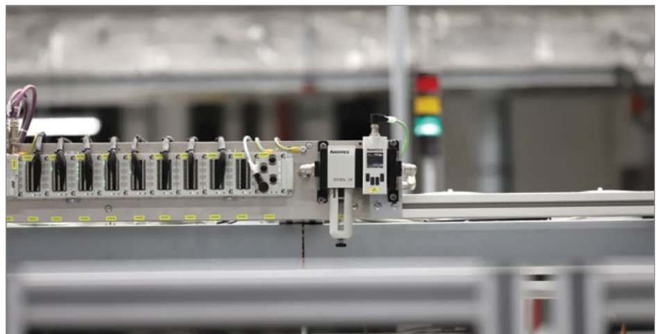
When installed on a facility's machines, the AVENTICS Series AF2 Flow Sensor empowers operators to monitor air consumption in pneumatic systems according to DIN ISO 50001 for energy management. Image courtesy of Emerson.
