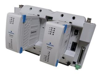
When paired with the Standalone Controller Software Toolkit software, the OCR3000 can operate as an independent, standalone application, in which a traditional Ovation network and database are not created.
