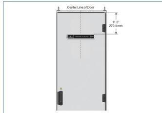
The nameplate insert is a Gravoply 2, 2-ply, black matte surface color with white core material that is 0.062" (1.57 mm) thick. The insert can be engraved with up to three lines of customersupplied cabinet and or equipment identification information. The recommended spacing for engraving is shown below.
