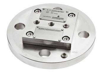
The LevelDatic Pneumatic 1:1 Converter PLT is used when measuring the hydrostatic pressure in tanks, where air feed into the tanks is prohibited or inadvisable because of liquid properties. The liquid level creates a hydrostatic counter pressure on the air flowing out from the pneumatic 1:1 converter which is used to determine the liquid level.
