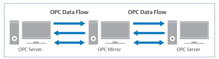
Redundant OPC Data Access servers provide highly reliable data transfer.
