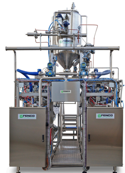
Figure 1. Rosemount magnetic flow meter installed in the new aseptic filling machine developed by Fenco
