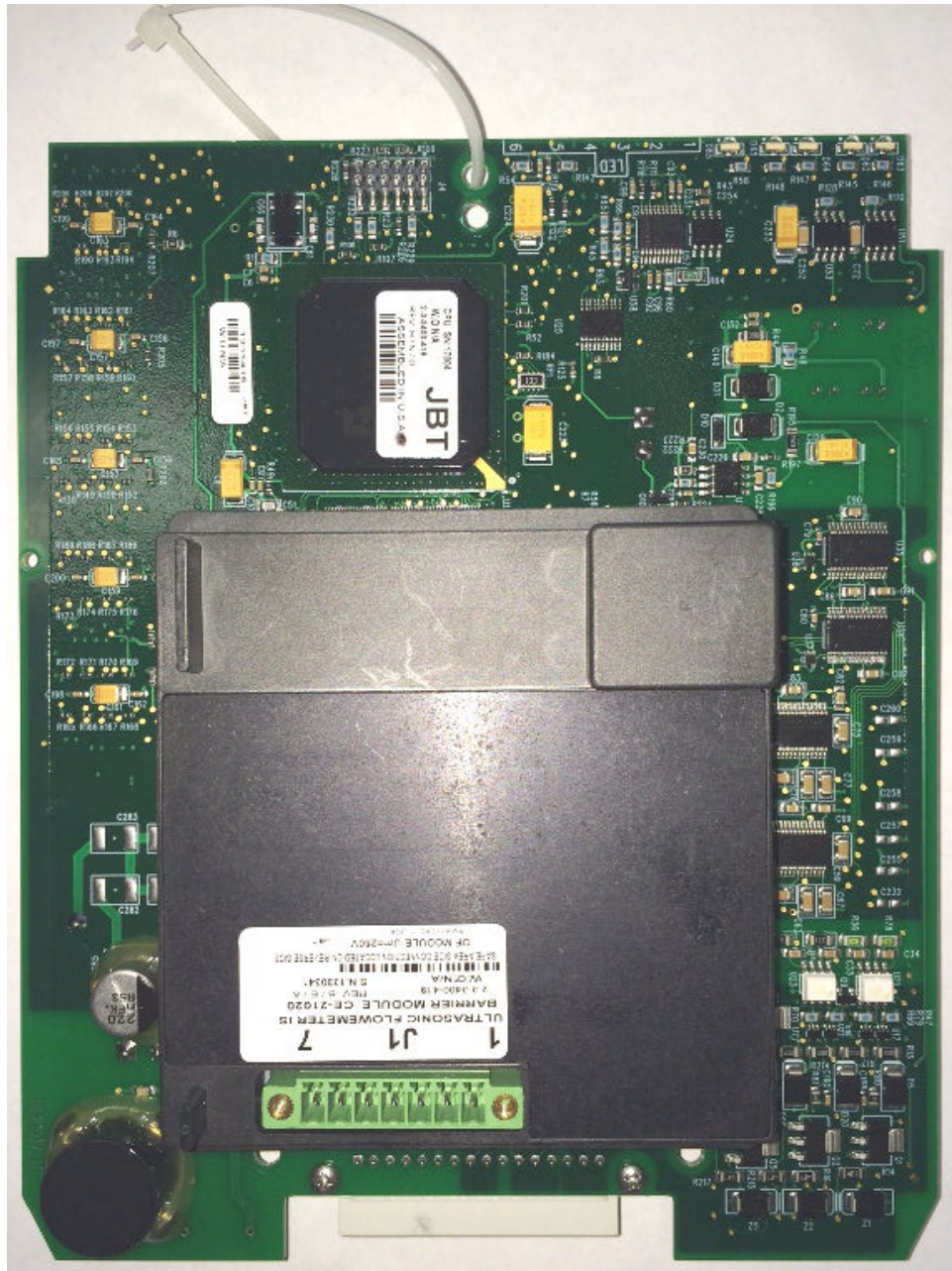
Figure 1-7: Mark III CPU Board with I.S. Barrier Board Piggy-Backed on CPU Board
