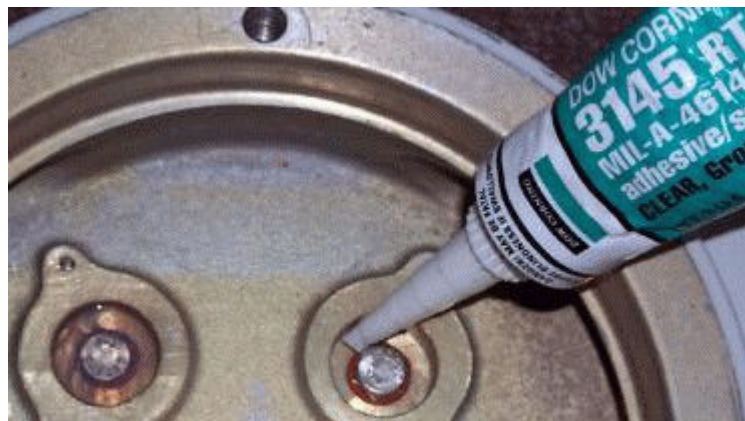
Figure 2-5: Apply RTV Sealant Around Bolts
