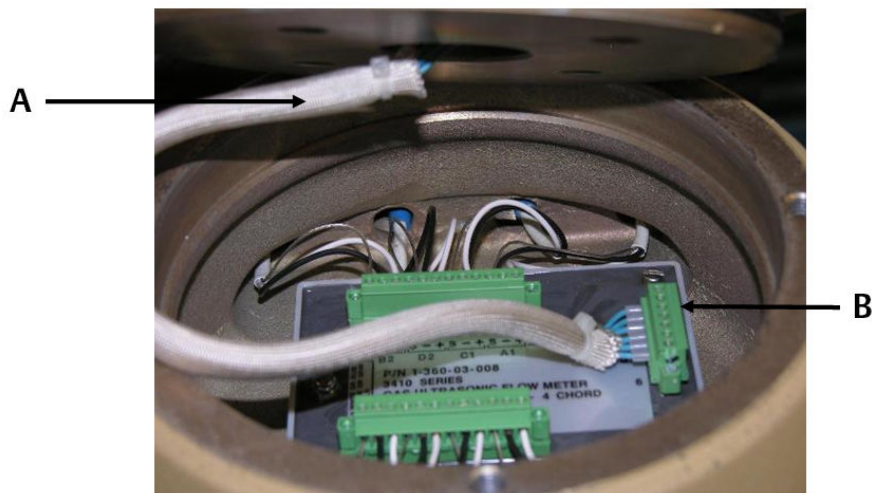
Figure 2-2: Remove Acquisition Cable and Module
