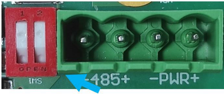
Figure 3-6: RS485 termination resistor
