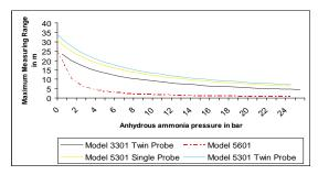
Measuring range in bar versus meters
