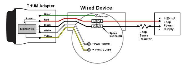
Figure 4. Wiring Diagram for THUM Adapter on a Two Wire Device
