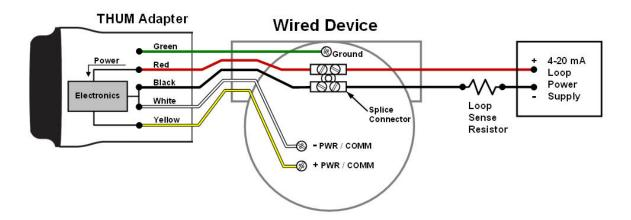
Figure 2. Wiring Diagram for THUM Adapter on a Two Wire Device
