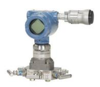
The THUM adapter connects to a HART wired device, collects the Hart data and then transmits that data over a Smart Wireless network. The THUM adapter is connected to the wired device both in series and in parallel on the 4-20 mA loop. Through the series connection the THUM adapter scavenges and stores energy to perform its basic functions. The parallel connection provides the THUM adapter with HART data communication.
