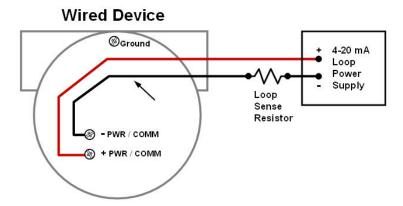
Figure 1. Wiring Diagram for Two Wire Device
