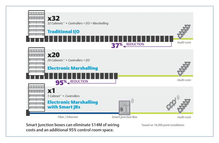
Although the project saves money in home-run multi-core cables, savings in wiring costs extend beyond the wires themselves to include engineering time, cable trays, conduits, and all the labor to lay the wire and connect each device. In addition, the redundant Fiber Optic Ethernet connection running from the field to the DeltaV system can simplify migration and modernization projects.
