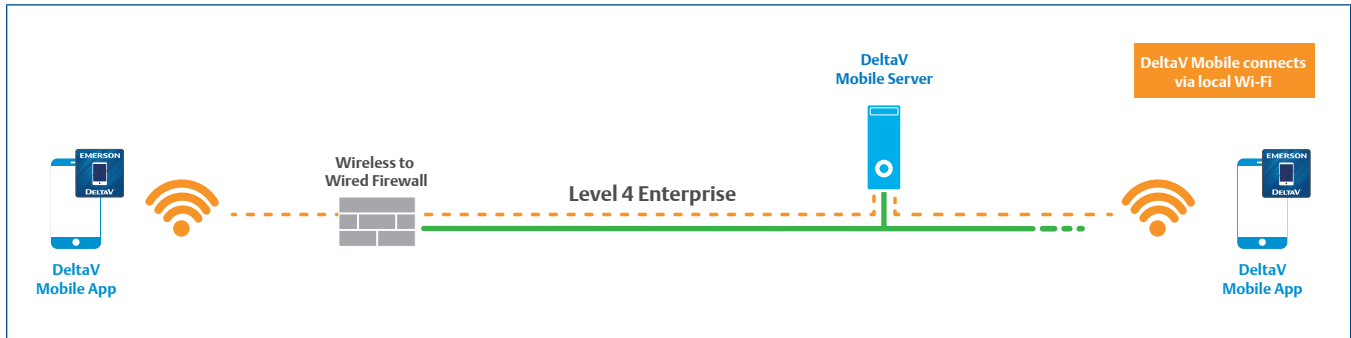
Figure 7. On-premise mobile connection in a 3-tier topology, either by direct Wi-Fi access to the Level 4 network or through a Firewall.
