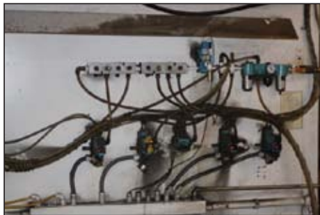
BEFORE: Pneumatic circuit on the load center machine consuming 75 cfm at idle.
