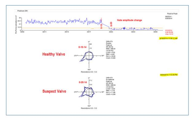
Let's first look at the trend value. Given the fact that we are dealing with a form of flow turbulence instead of impacting, what we notice is that the amplitude actually decreases when a value is not properly sealing. This is due to the fact that the Delta Pressure is less across an improperly functioning value, the usual "surge" of gas as the value opens and closes is substantially reduced.
