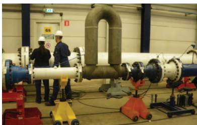
Figure 5. NMI Euroloop Test Setup for Large Coriolis Sensor
