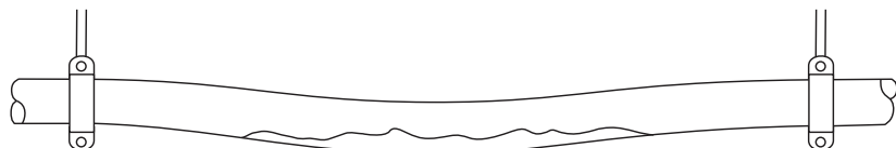
FIGURE 2.8 Water hammer can result from accumulation of condensate in a sagging steam main
