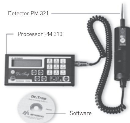
Photo shows system manufactured by Miyawaki that combines testing of the trap with data storage and reporting
